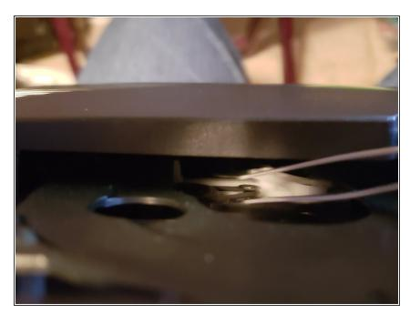
There will be a gap in the middle of the CD/DVD tray. You will see 2 pulleys with a rubber belt. Use tweezers to carefully take the belt out.
