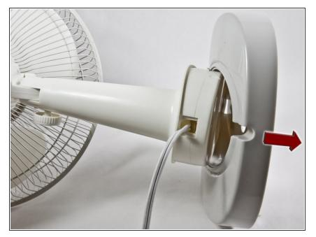
After the base has separated more it will be easy to fully remove it. Continue pulling the back edge of the gray base support, rotating it around the front tab until it comes off completely.
