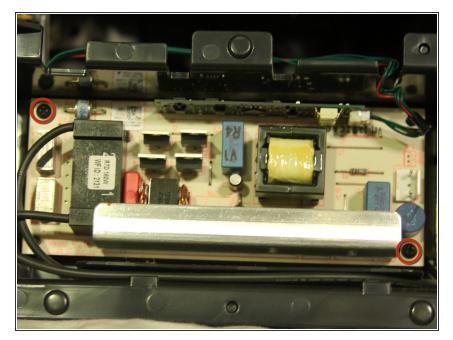
Remove two 14 mm Phillips #0 screws securing the lamp ballast to it's housing.
