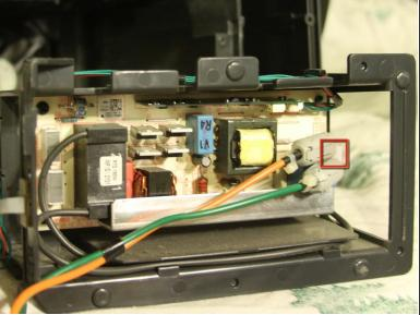
Disconnect the orange and green power connection from the lamp ballast by holding the white tab
