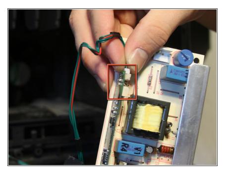
Disconnect the green and red main board connection from the lamp ballast by gently pulling straight back out of the socket.
