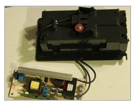
Remove one 10 mm Phillips #1 screw from the back of the lamp ballast housing.
