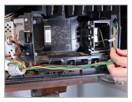
Pull up and unsecure the orange and green power connection wires that are being held down by the white clamps and black cable hooks.
