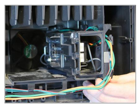
Pull straight back on the lamp ballast housing to remove it from the television.
