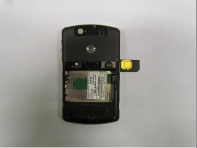
Remove the existing SIM card (if applicable) by applying little pressure with one finger and dragging it until the card is completely out.
