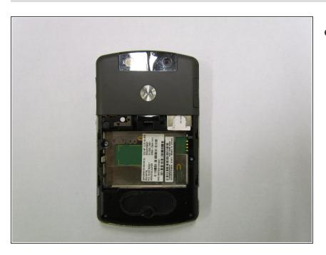
Insert the new SIM card into the card reader with the chamfered edge in the upper left corner.
