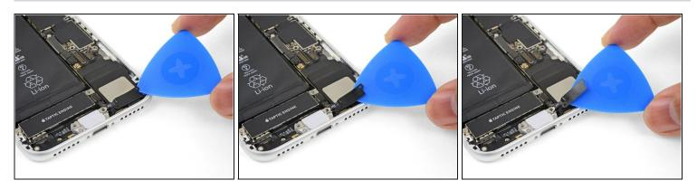
Gently slide an opening pick between the antenna flex cable and the top of the speaker.
