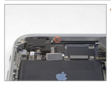
• Remove the 1.4 mm Phillips screw securing the antenna component to the top of edge of the case.
