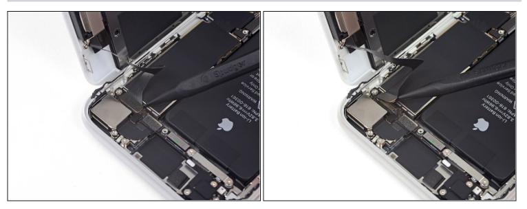
• Use the point of a spudger to disconnect the front panel sensor assembly connector.
