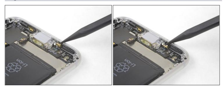
• Use the point of a spudger to gently pry the battery-side microphone free from the adhesive securing it in place.
