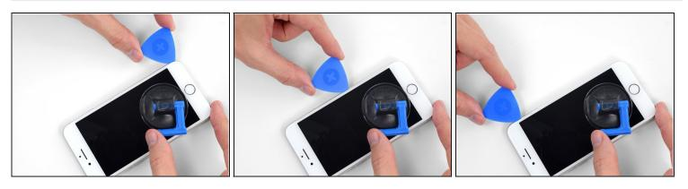
Re-insert your tool at the lower right corner of the iPhone, and slide it around the corner and up the right side of the phone to separate the adhesive.
