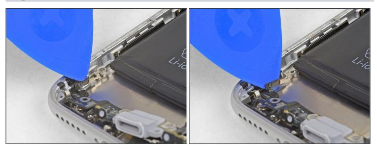
• Slide an opening pick between the left edge of the case and the remaining adhered section of the Lightning assembly.
