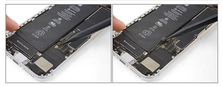
• Use the point of a spudger to pry up and disconnect the diversity antenna flex cable from the logic board.
