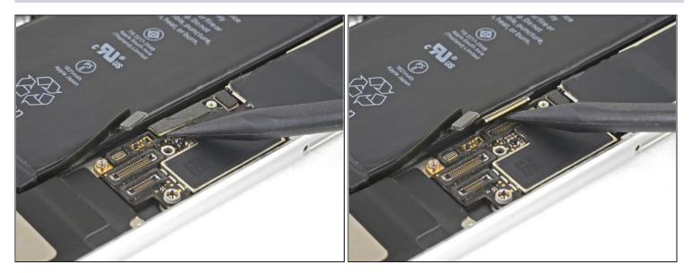
• Use the point of a spudger to pry up and disconnect the Lightning connector cable from the logic board.
