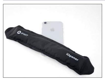
• Apply a <u>heated iOpener</u> to the bottom of the phone, angling it as shown. This will help loosen the flex cable adhesive.
