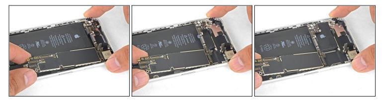
• Grasping it by the edges, lift the logic board near the battery connector and remove it.
