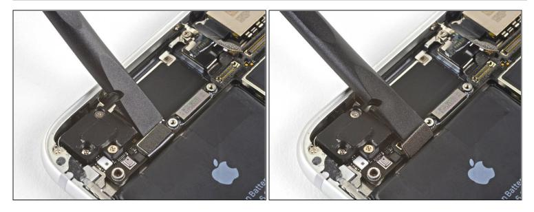
• Use the flat end of a spudger to pry the upper cable connector up from its socket.
