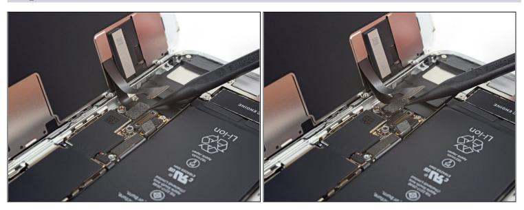
• Use the point of a spudger to disconnect the second lower display cable.
