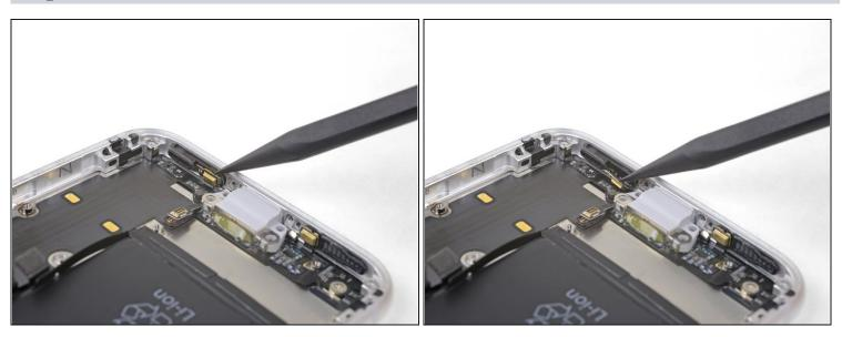
• Use the point of a spudger to gently pry the logic-board-side microphone free from the adhesive securing it in place.
