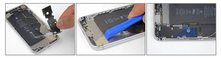
• Remove the Lightning connector assembly.
