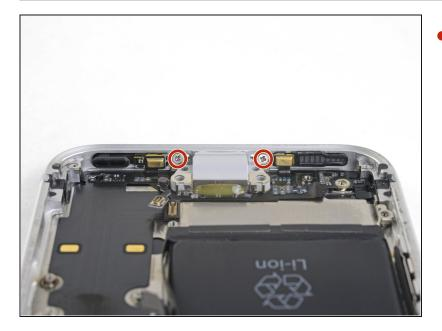
• Remove the two 1.4 mm Phillips screws securing the Lightning port to the bottom edge of the phone.
