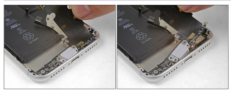
• Gently pull the Lightning connector out of its hole on the rear case.
