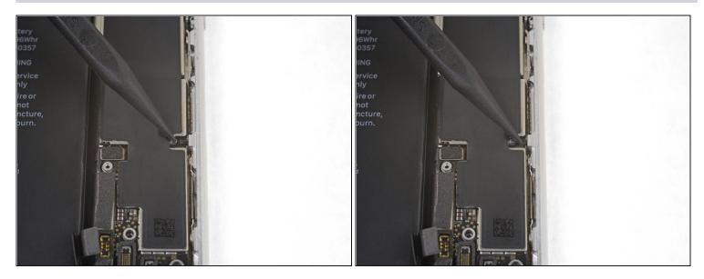
• Use the point of a spudger to move the SIM card eject plunger out of the logic board's way.
