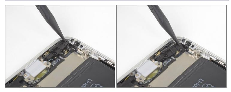
• Gently push the barometric vent in the direction of the battery to separate the adhesive securing the vent to the bottom edge of the iPhone.
