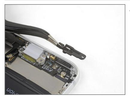
• Remove the barometric vent.
