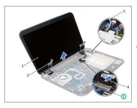
Peel the tape that secures the display cable to the system board and then disconnect the display
