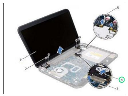
Route the display cable through the routing guides and connect the display cable to the connector on the system board.
