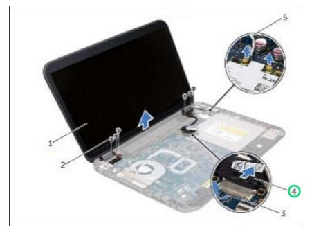
Make a note of the display cable routing and remove the cable from the routing guides.
