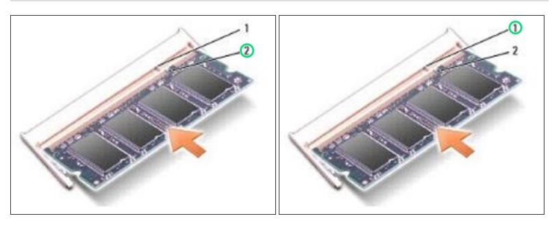
• Align the notch in the module edge connector with the tab in the connector slot.
