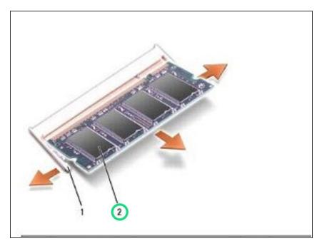
Remove the module from the connector.
