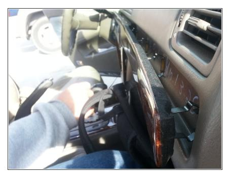
Using a panel tool or long flat head screwdriver, pry the wood grain trim off and release the clips. Be careful on the thin sections below the head unit as to not snap the trim.
