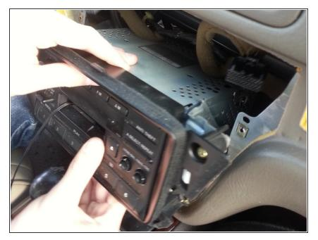
Pull the head unit straight out gently until the two wire harnesses are exposed.
