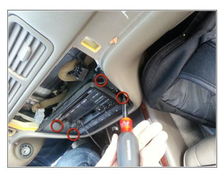
• Unscrew the four screws from the sides of the deck, circled here.
