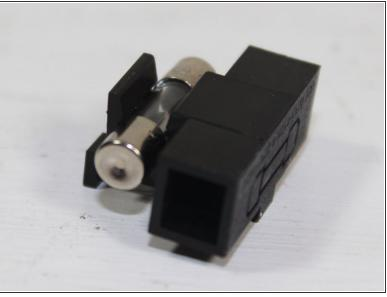
Remove the blown exposed fuse and replace it with the enclosed fuse. If there is not an extra
