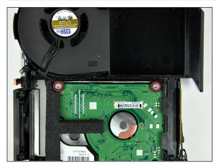
Remove the two Phillips screws securing the bottom of the hard drive to the internal frame.
