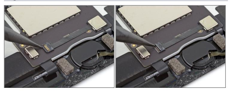
• Use the point of a spudger to lift the flap on the ZIF connector that secures the cable.
