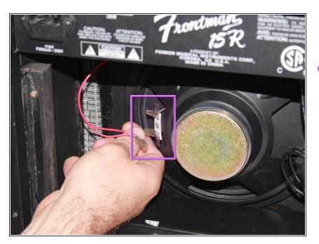
Label and unplug the two red wires connecting the mounting bracket to the speaker by pulling them off the nodes.
