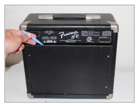
Once the screws are out, use a plastic opening tool or spudger to pry the top of the back panel open.
