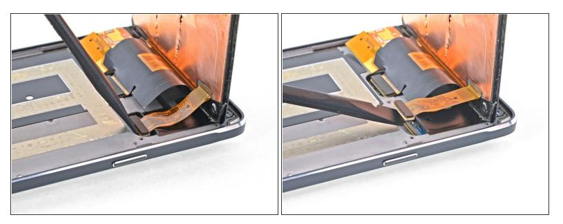
Use the flat end of a spudger to pry the display cable connector straight up and out of its socket.
