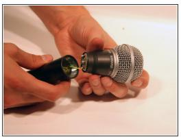
Grab the microphone base with one hand. With the other hand, grab just below the grille (the collar). Twist the collar clockwise to loosen it.
