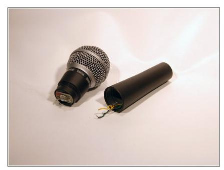
insulation, strip the broken wire. See wire stripping guide.
