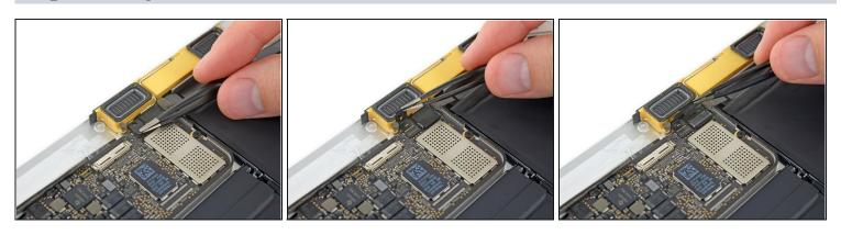
• Use tweezers to peel up the tape covering the two ZIF connectors—one for the right speaker cable, and one for the audio jack board cable.
