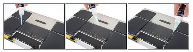
• Lay the lower case assembly down flat, and apply adhesive remover to the two middle battery cells—at each side, and along the front edge (opposite the logic board area).
