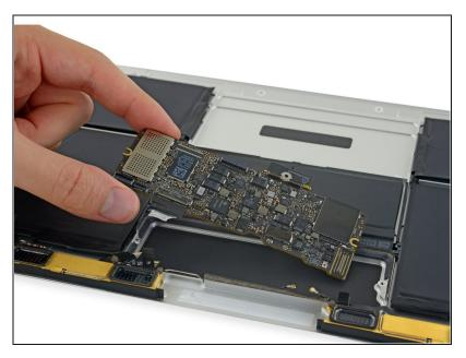
• Remove the logic board.
