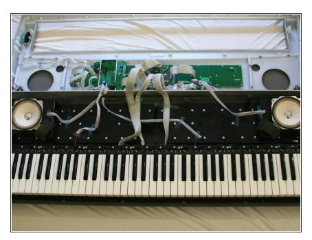
Locate the main circuit board in the middle of the detached face plate.
