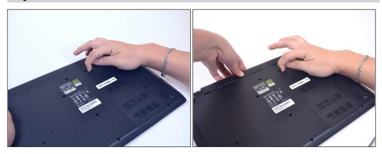
Slide the locking latch to the right and hold while pulling the battery out with your other hand.
