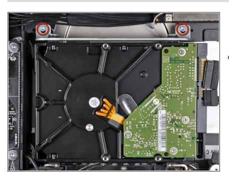
Remove the two T10 Torx screws securing the upper hard drive bracket to the outer case.
