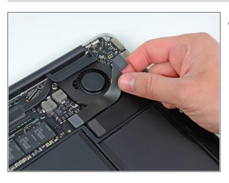
Carefully peel the I/O board cable from the top of the fan.
