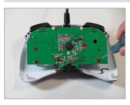
Locate the four 8.3 mm Phillips screws on the circuit board and remove them.
