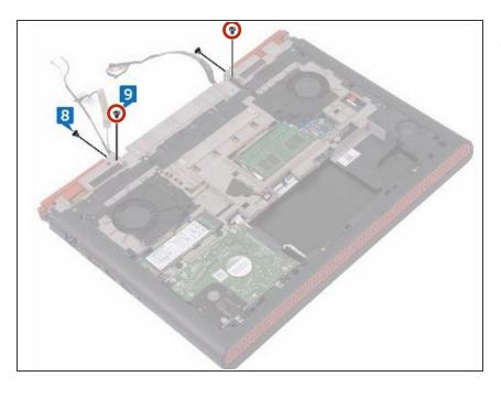
Replace the two screws (M2x3) that secure the display assembly to the computer base.
