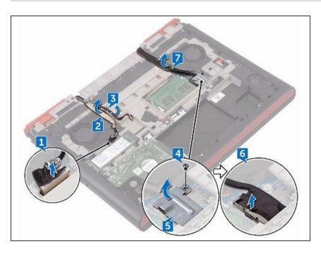
Using the pull-tab, disconnect the display cable from the system board.
