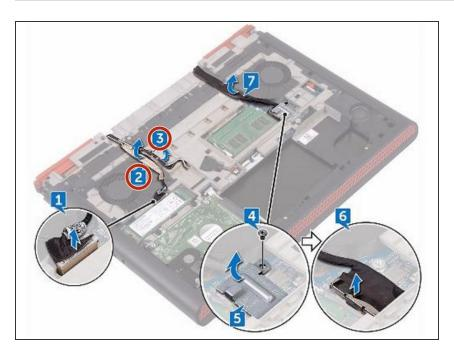
Connect the display cable and camera cable to the system board.
