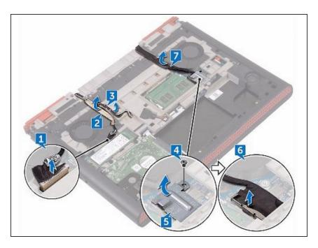
Peel off the display cable from the computer base.
