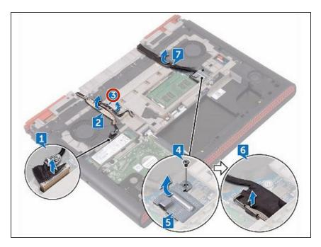
Remove the antenna cables from the routing guides on the computer base.
