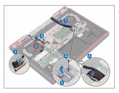
Peel off the camera cable from the computer base.
