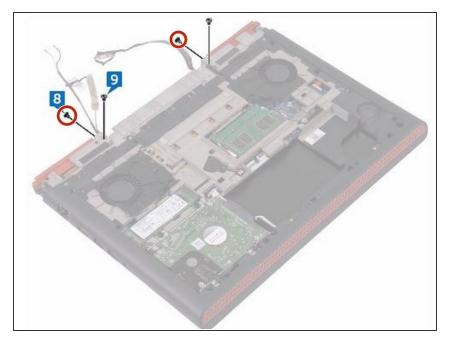
Remove the two screws (M2.5x5) that secure the display assembly to the computer base.
