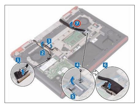
Adhere the display cable and the camera cable to the computer base.
