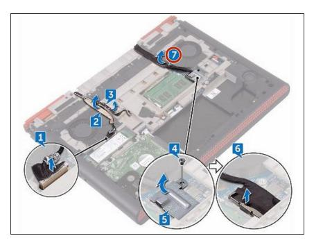
Lift the display-cable bracket off the system board.
