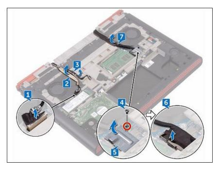
Align the screw hole on the displaycable bracket with the screw hole on the system board.
