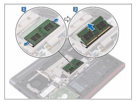
Align the notch on the memory module with the tab on the memorymodule slot and slide the memory module firmly into the slot at an angle.
