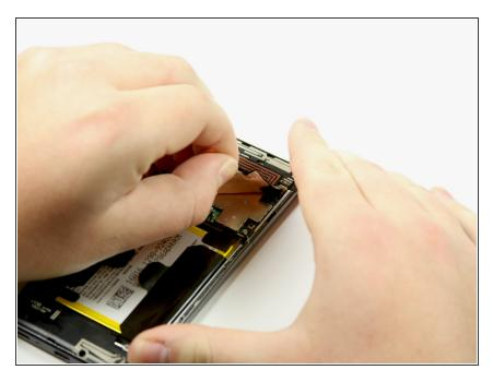
Peel back the RAF antenna.
