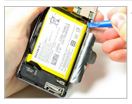
Use a plastic opening tool to get under the battery and pry it up.
