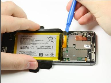
Use a plastic opening tool to pry up the orange battery connector that is directly above the battery in the center of the phone.
