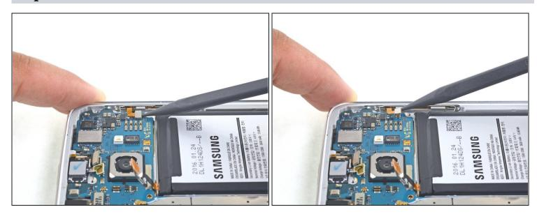
• Use a pointed end of a spudger to disconnect the volume button cable.
