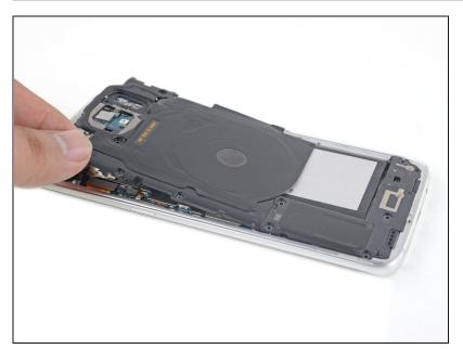
• Lift and remove the wireless charging coil from the phone.
