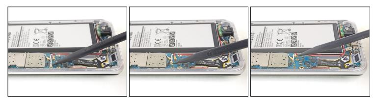
• Use the pointed end of a spudger to disconnect the red and white antenna cables.
