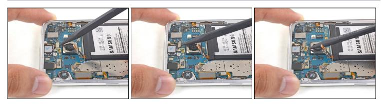
• Use the pointed end of a spudger to disconnect the front-facing sensory array cables.
