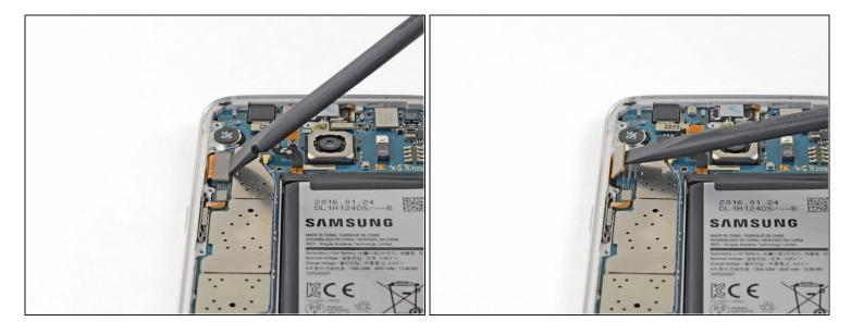
• Use the flat end of a spudger to disconnect the display cable.
