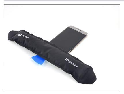
With the opening pick in place, apply a heated iOpener to the top edge once more in order to soften the adhesive.
