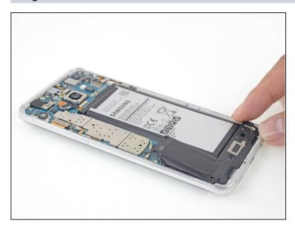
Lift and remove the loudspeaker from the phone.
