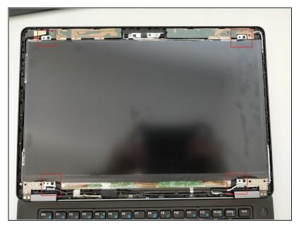
• Remove the 4 Philips screws securing the panel.
