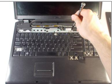
Remove the four 3mm Phillips #0 screws.
