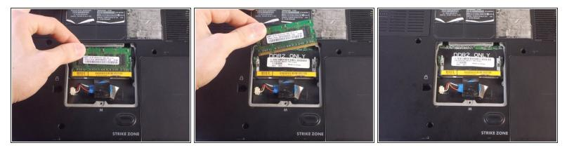
• Lift the RAM chip up and out of the slot.
