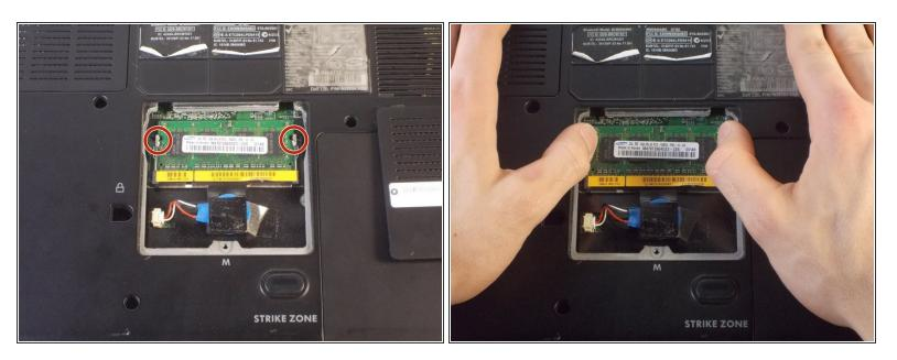
Dislodge the RAM from its slot by pushing outwards on the retaining clips.
