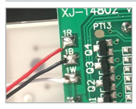
Carefully add solder to each area where a connection will be made on the new board. This will make it easier to actually create connections.
