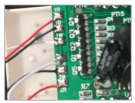
Solder all of the components back onto the new board being very careful to not let any of the connections touch, which would cause more errors.
