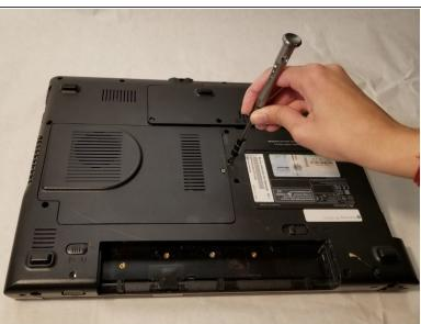
Using the Phillips #1 screwdriver, remove the four 6mm screws on the back of the laptop.
