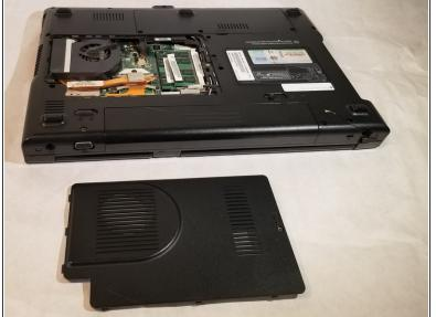
Insert the plastic prying tool and pry the back panel off starting at an edge and moving your way around it. To reassemble your device, follow these instructions in reverse order.
