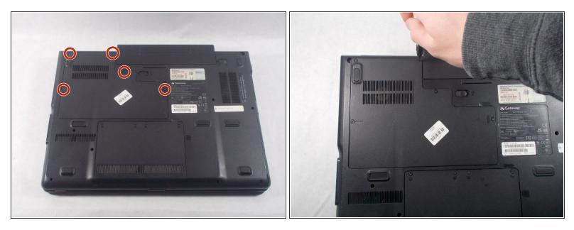
Turn your laptop upside down and remove the five Philips #0 (5mm) screws for the cover of the Heatsink.
