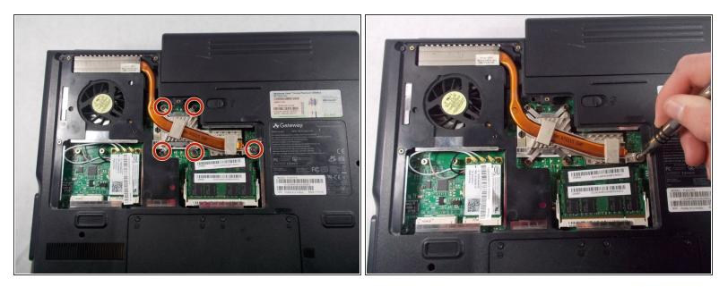
Remove the five Phillips #0 (5mm) screws around the Heatsink.
