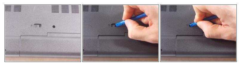
On the back of the laptop, there is a sliding lock. Push the slider and the battery will unlock
