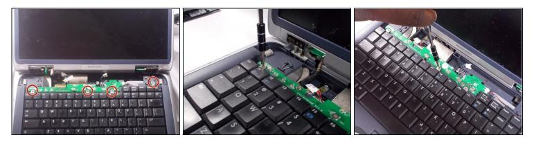
• Remove the four 4.0 mm Phillips #0 connecting the keyboard to the frame
