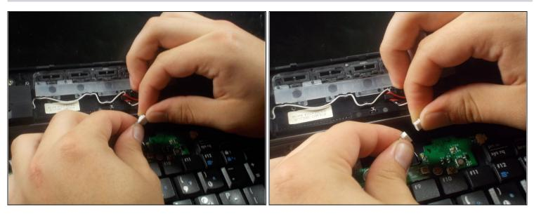
• Remove the wire connection by gently pulling on the fuse and connection itself.
