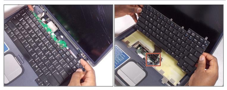
• Gently lift the keyboard up from the frame so that you can see the ribbon still connected.
