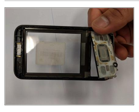
If it is the actual main screen panel control buttons that need to be replaced, grab the front panel as seen in the picture and push from the outside in with little pressure as if you were regularly trying to use the button.
