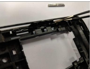
Use a pair of tweezers to grab hold of each button on an edge from inside of the casing and pull out to remove.
