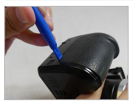
Insert the plastic opening tool underneath the rubber on the bottom corner.
