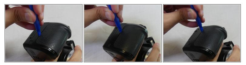
• Slide the plastic opening tool along the perimeter of the rubber grip to unbind the glue.
