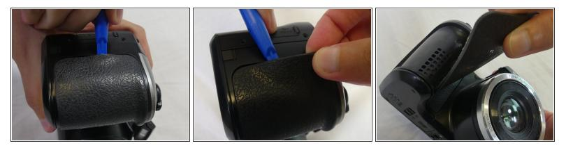
Pry upwards until you can grip the rubber enough to pull off.
