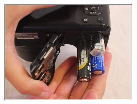
• Remove the batteries.
