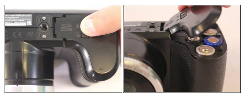
• Press down on the battery cover and slide outwards to open.
