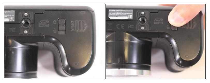
• Slide switch to open lock position.
