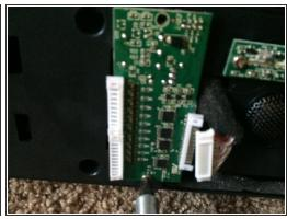
Remove the two screws holding the led controller in place.
