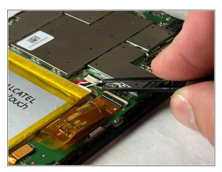
Disconnect battery by pulling up on the ZIF connector with precision tweezers for safety.
