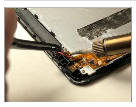
Solder the wires off of the motherboard with a soldering iron while holding the wires with the precision tweezers. For information on how to solder safely and correctly go to this link: <u>How To Solder and</u> <u>Desolder Connections</u>
