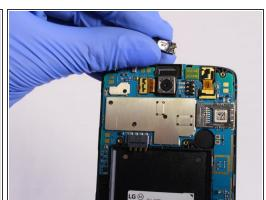
Remove the speaker by using the Spudger.
