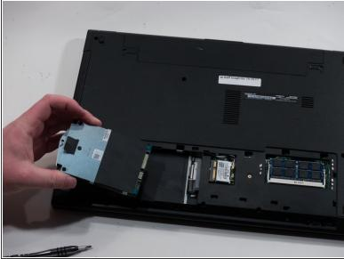
Pull the black tab up and to the left to completely remove the hard drive.
