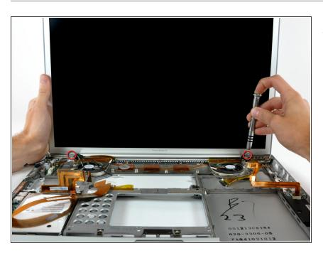
While supporting the display with one hand, remove the last two T6
