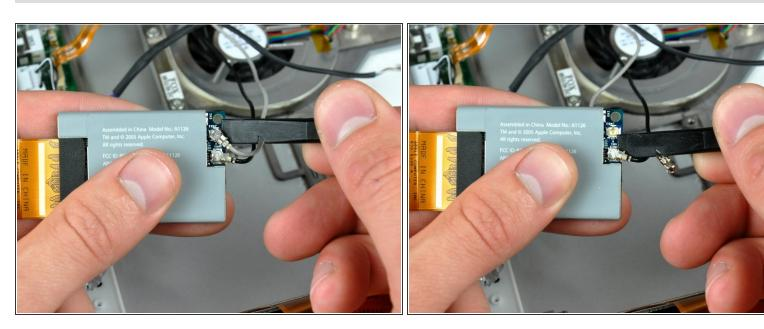
Use the flat end of a spudger to pry both antenna connectors off the AirPort/Bluetooth board.
