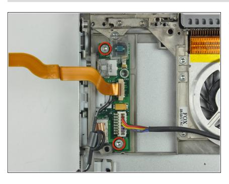
Remove the two T8 Torx screws securing the DC-in board to the lower case.
