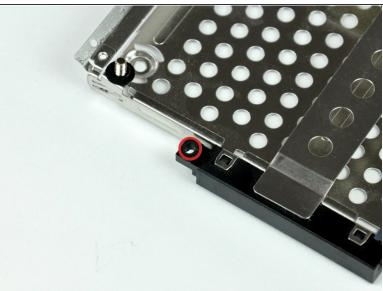
When reinstalling your PC card cage, be sure to insert the post sticking up from the PC card release button into the hole in the black plastic release mechanism on the PC card cage.
