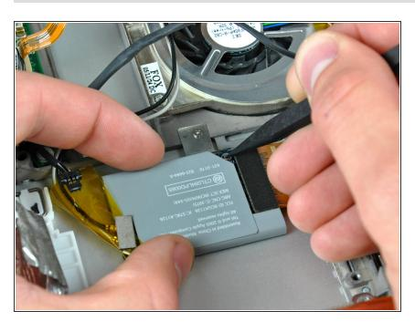
Use the tip of a spudger to press the metal pressure connector down through the hole in the AirPort/Bluetooth board and lift it out from the lower case.
