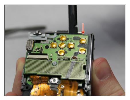
Insert the flat end of a plastic spudger underneath the motherboard and twist. This will disconnect the board from the device and allow it to be removed.
