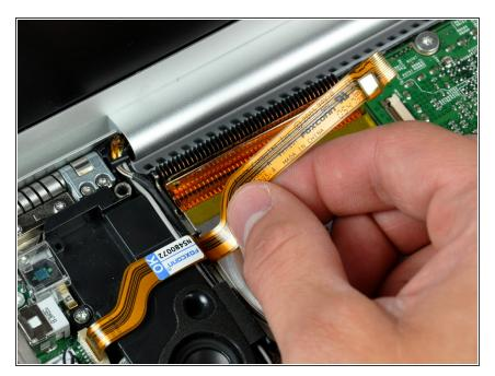
• Peel the DC-in cable off the adhesive securing it to the lower case.
