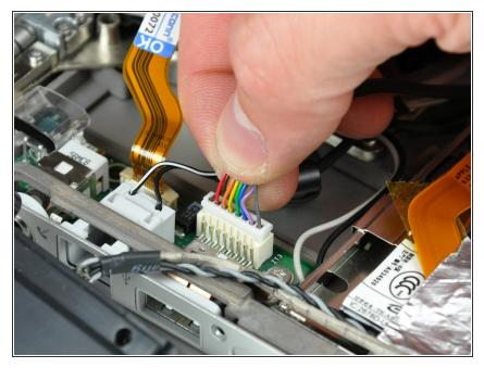
• Pull the DC power cable connector straight up off the DC-in board.
