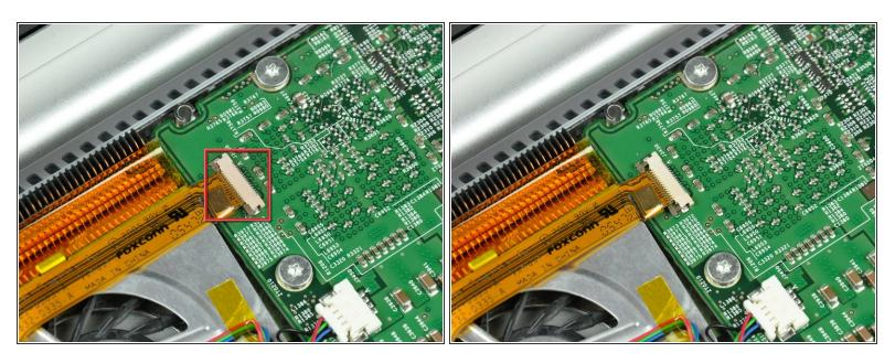
• Use your fingernails or the tip of a spudger to separate the ZIF cable lock from its socket.
