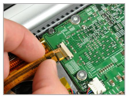
• Pull the DC-in cable out of its socket.
