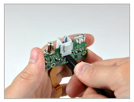
Use the flat end of a spudger to continue removing the RJ-11 board away from the DC-In board.
