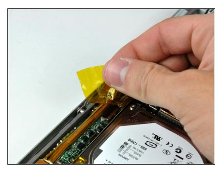
• Remove the strip of tape covering the speaker cables.
