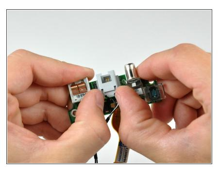
Use your thumbs to slide the RJ-11 board slightly away from the DC-In board.
