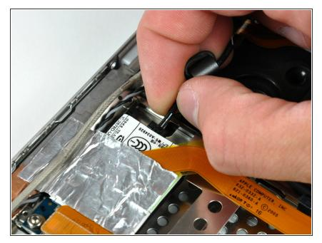
• Disconnect the RJ-11 cable from the modem.
