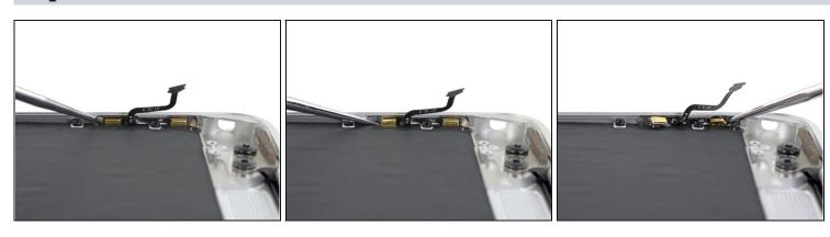
• Use a fine-tip probe or pick to gently peel the dual microphone assembly away from the case.
