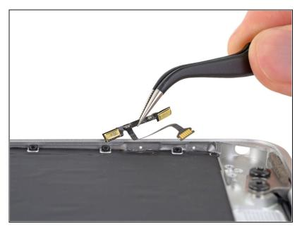
Remove the dual microphone assembly.
