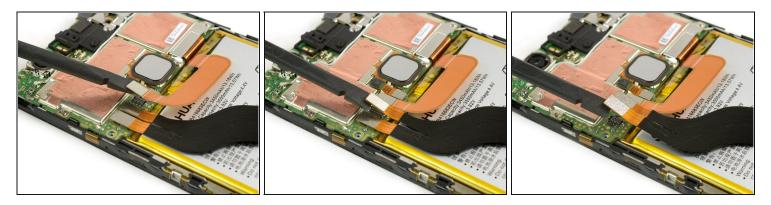
Use the flat end of a spudger to disconnect the three flex cables.
