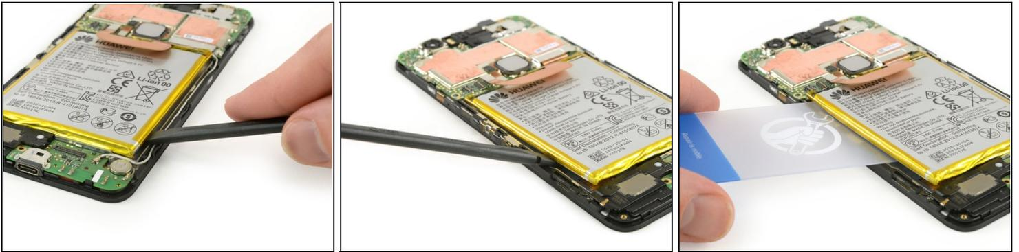
**⚠ Warning: do not insert the spudger or plastic card too deep underneath the battery. The display cable runs underneath the battery.**
