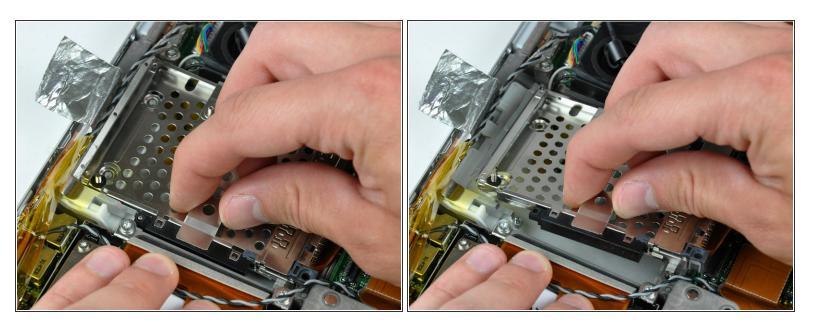
Lift the PC card cage by its center piece and maneuver it out of the lower case.
