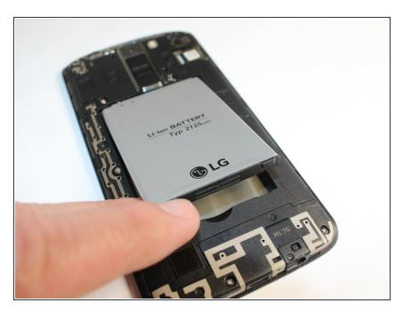
Remove the battery from the phone by lifting up on the bottom end of the battery.
