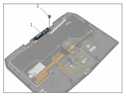
Align the screw hole on the status-light board with the screw hole on the palm-rest assembly.
