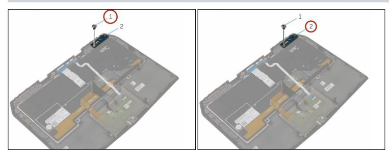
Remove the screw that secures the status-light board to the palm-rest assembly.
