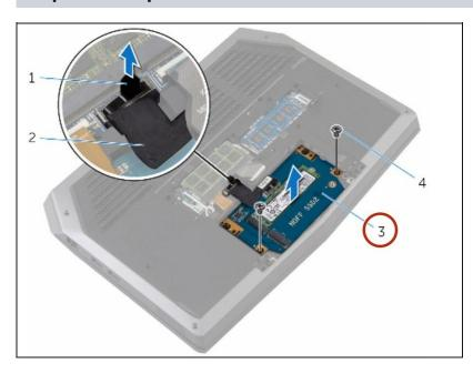
Replace the screws that secure the solid-state drive assembly to the computer base.
