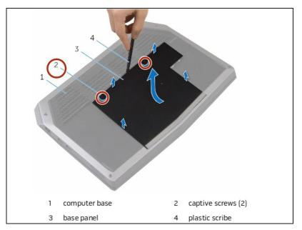
Loosen the captive screws that secure the base panel to the computer base.
