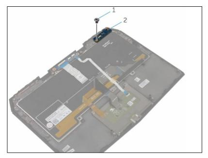
Replace the screw that secures the status-light board to the palmrest assembly.
