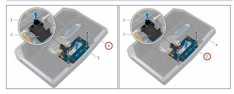
• Remove the screws that secure the solid-state drive assembly to the computer base.
