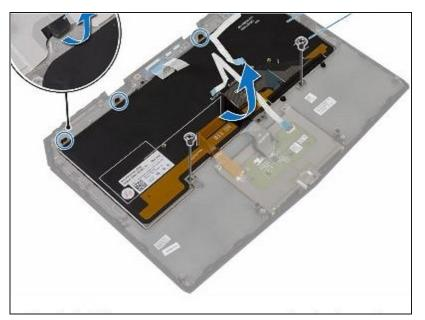
Align the screw holes on the NEW keyboard with the screw holes on the palm-rest assembly.
