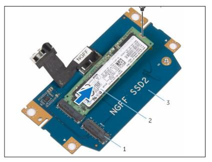
Slide the **NEW** solid-state drive into the slot on the solid-state drive assembly.
