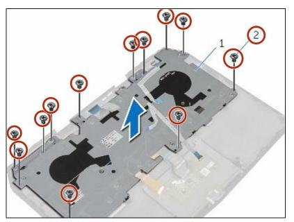
Remove the screws that secure the keyboard bracket to the palmrest assembly.
