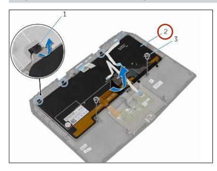
Slide and lift the keyboard, along with the cables, off the palm-rest assembly.
