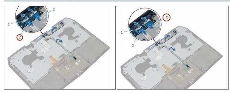
Peel the touchpad cable and status-light cable off the keyboard bracket.
