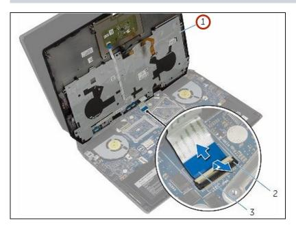
Lift the palm-rest assembly off the computer base.
