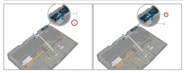
Slide the status-light board cable into the status-light board connector and press down the latch to secure the cable.
