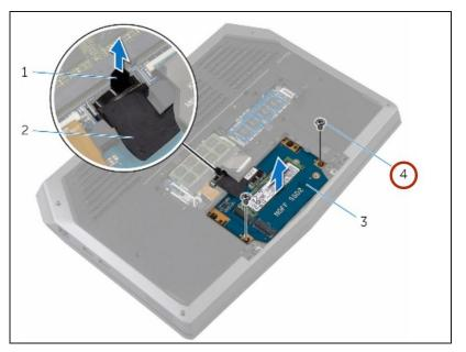
Remove the screw that secures the solid-state drive to the solidstate drive assembly.
