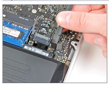
Use the flat end of a spudger to pry the sleep sensor/battery indicator connector up from its socket on the logic board.
