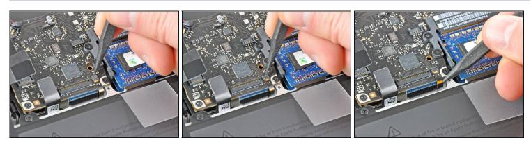
• Use the tip of a spudger or your fingernail to flip up the retaining flap on the keyboard backlight ribbon cable ZIF socket.
