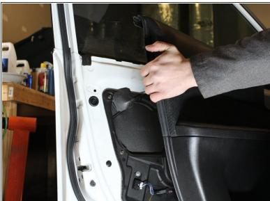
Lift the door panel up and out to remove.
