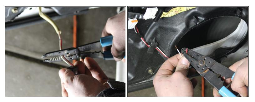
Cut and strip the wires that were connected to the speaker.
