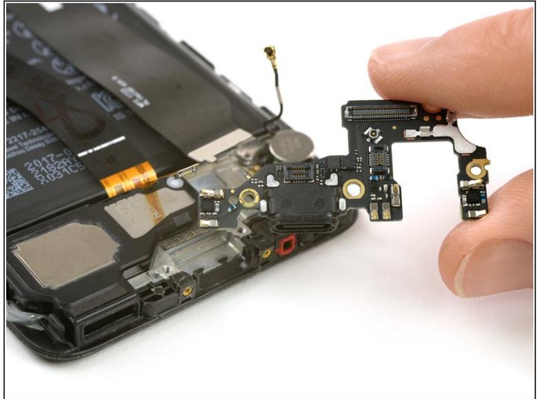
**!** Do not damage any components sitting on the charging board while removing it.
