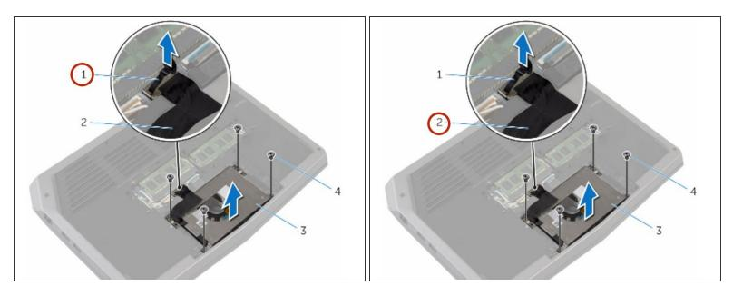
• Using the pull tab, disconnect the hard-drive cable from the system board.
